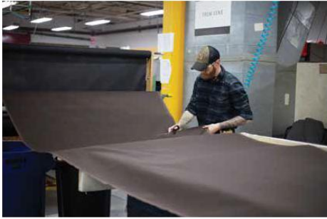
Preparing fabric for pattern cutting on the laser cutter.
