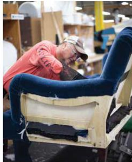
Skilled artisan upholstering fabric to the wooden frame.
